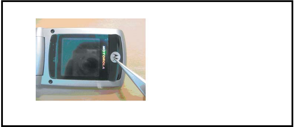
Figure 28. Replacing the Screw Cover and Screw Cap
