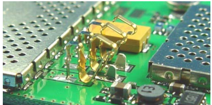
Desolder all pins and clean the pads.
