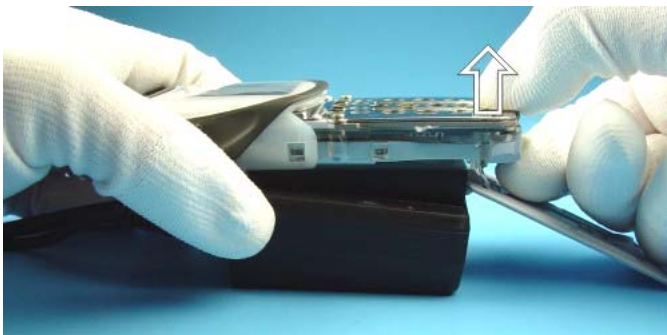
When removing the Flash Adapter, always start from the bottom side of the unit.
