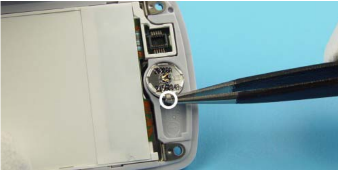
Remove Earpiece. Note the guiding pin when assembling.
